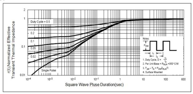
Figure 7. Typical Effective Transient Thermal Impedance, Junction-to-Ambient
